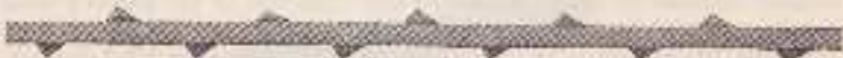
Fig. 3 Looking from the back of a saw. This shows how the teeth, when set, extend beyond the edge of the blade.
