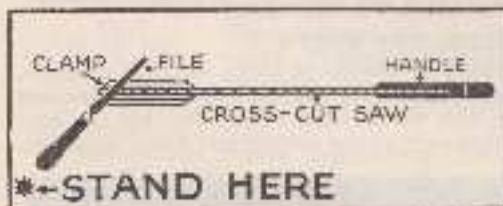
Fig. 8—First position for filing hand saw for cross-cutting.
