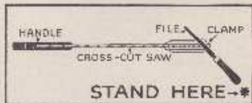
Fig. 9—Second position for filing cross-cut saw.
